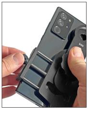
2. Set the height of the phone clamp (C) to securely hold your smartphone model in the adapter by turning the clamp adjustment knob (E), turning clockwise lowers the clamp, turning anti-clockwise raises the clamp.
