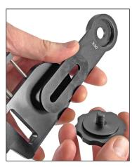
7. To remove or change the opticsrail with a different version (sold separately) unscrew the locking wheel totally (A) so that the opticsrail is released. Replace with your chosen opticsrail and insert the locking wheel, turn clockwise to tighten.
