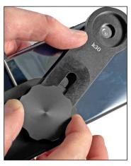
**4.** Once alignment has been achieved, secure the Opticsrail (I) by turning the locking wheel (A) clockwise until it is secured in place.
