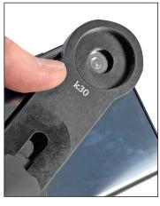
3. Loosen the locking wheel (A) and then rotate the Opticsrail (I) so that the hole sits central over the lens of your smartphone camera. If your smartphone has multiple lenses - simply align the hole with the lens you want to use.
