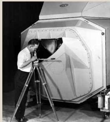
A Farrand technician (left) tests the Infinity Display system Al Nagler designed for the Lunar Module simulator (middle). During the test, the triangular lens opening shown fit against one of the module's windows. In the schematic of the Infinity Display (right), the small triangular "compressor
