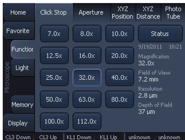
Fig. 21 Control Panel Showing Preset Magnifications
