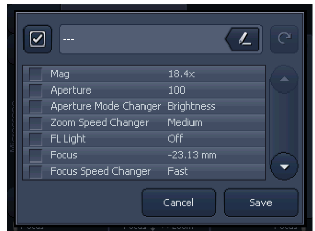
Fig. 42 Selection Menu for Saving Device Settings and for Assigning Names to Device Settings
