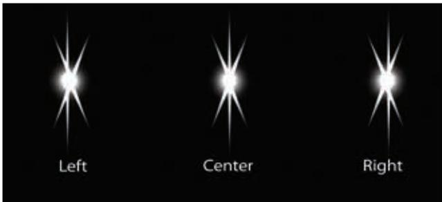
**Figure 5.** As the telescope's focus is adjusted, the middle spike of the diffraction pattern moves left and right of center of the “X” formed by the other two diffraction spikes. Adjust focus until the middle spike is exactly centered in the X; that's when precise focus has been achieved.
