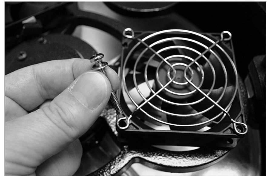
Figure 2. Place a washer on each mounting screw, then insert the screw through the wire cover and fan and into the threaded hole in the metal support cell. Tighten all four screws to secure each fan in place.
