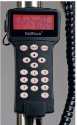
Far left: To help with balancing the mount, the right ascension and declination drives have gear switches (arrowed) that release the worms from their worm wheels. Near left: The hand control has variable-brightness illumination for the display and buttons. The illumination automatically turns off during periods of inactivity, but returns the moment any button is pressed.
