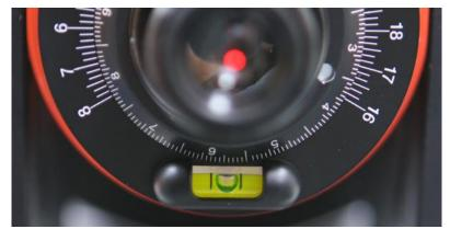
③ Turn the RA axis and make adjustments so that the level mounted on the polar axis telescope becomes level.
