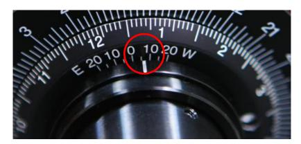
① Move the longitude reference line of the polar axis telescope by as much as the longitude difference of the surveyed area based on longitude 135°E. Move toward W by 8.5 for Seoul and toward W by 5.5 for Busan.
