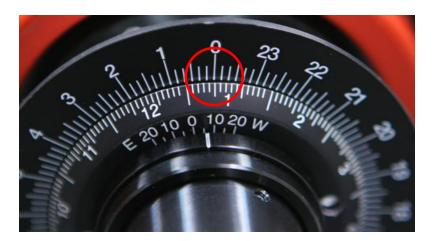
② Turn the eyepiece of the polar axis telescope and set the date ring and the time ring to the current date and time, respectively. One graduation of the date ring indicates 2 days. The photo shows the date and time set as of 0 o'clock (12:00 at night) on January 10.
