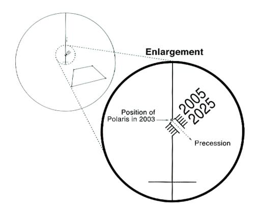
④ Turn on the lighting system of the polar axis telescope and introduce Polaris into the field of vision of the polar axis telescope through the use of the equatorial mount's altitude controller and the azimuth controller. Since the position of Polaris changes slightly every year according to precessional motion, position according to year.
