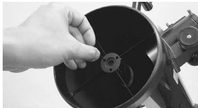
Figure 16. Adjust the tilt of the secondary mirror by loosening or tightening the three alignment set screws with a 2mm hex key.
