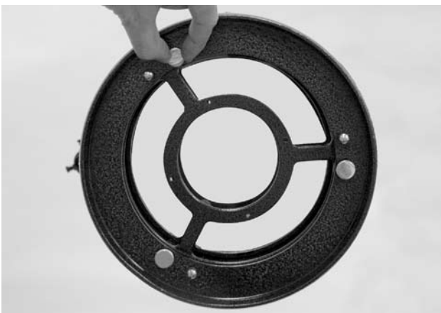
Figure 18. The tilt of the primary mirror is adjusted by turning one or more of the three larger thumbscrews.
